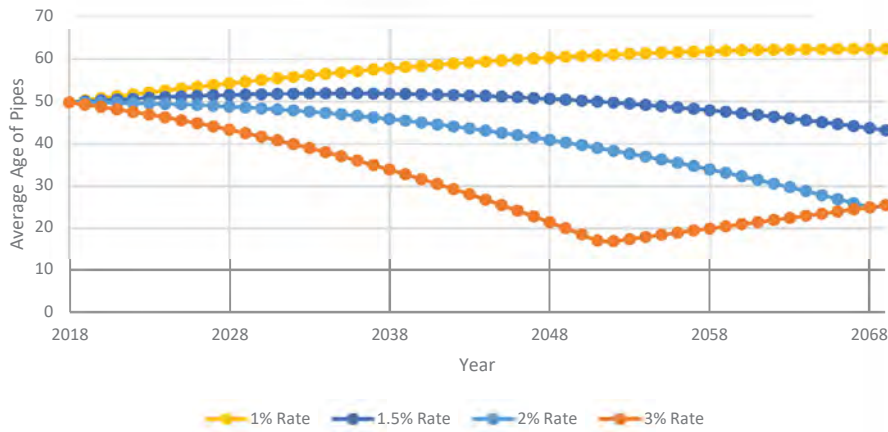
Figure 14: Average age of pipelines under 1-3% replacement programs
